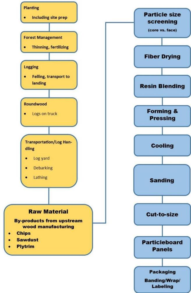
Figure 1: Cradle-to-gate product system for particleboard
