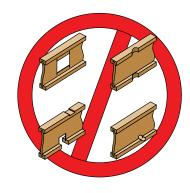
**Never** drill, cut or notch the flange, or over-cut the web. Holes in webs should be cut with a sharp saw. For rectangular holes, avoid over-cutting the corners, as this can cause unnecessary stress concentrations. Slightly rounding the corners is recommended. Start the rectangular hole by drilling a 1"-diameter hole in each of the four corners and then make the cuts between the holes to minimize damage to the I-joist.
