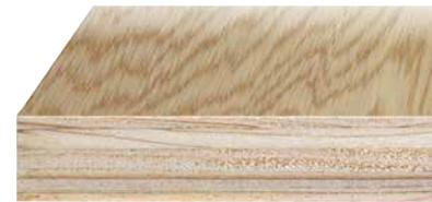
**HARDWOOD CROSSBAND VENEER:** Combines the smooth finish of a hardwood veneer crossband beneath the face and back with the strength and durability of Western softwood veneer inner plies. Together they create an excellent hardwood plywood panel that is smoother and has less potential for core telegraphing. Weighs 65 pounds.
