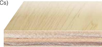
**MULTI-PLY:** A premium-quality multi-layer veneer core panel constructed of nearly void-free, uniform birch veneer. This all-hardwood core produces an attractive, uniform edge for those requiring an exposed edge finish. Often used for drawer sides, this panel is also preferred for its consistent cutting performance. Weighs 80 pounds.
