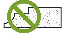
Dry film build of top coat - minimum 2.5 mils. Reminder: All paints will draw away from a sharp edge or corner, regardless of what is being painted: metal, plastic, lumber, plywood and Medex. Because the paint is very thin on this area, any expansion and contraction resulting from ambient changes will cause the paint to crack.
