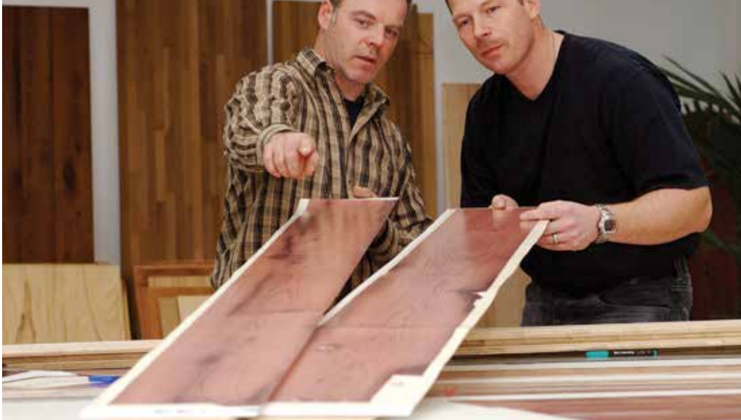
Manually laying up a panel design with plotter prints of lumber scans.
