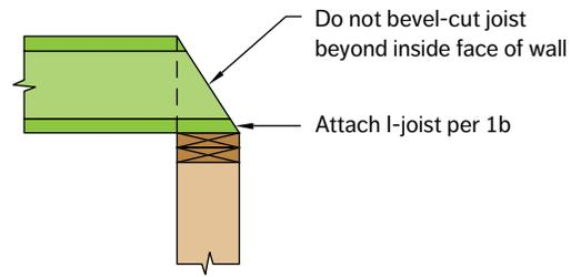
**Note:** Blocking required at bearing for lateral support, not shown for clarity.
