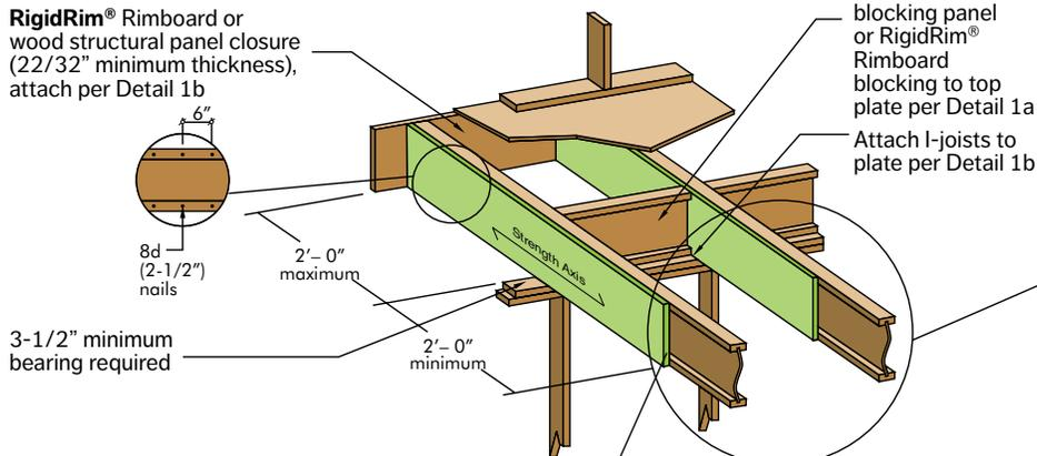
APA RATED SHEATHING 48/24 (minimum thickness 22/32"), or RigidRim Rimboard, required on sides of I-joist. Depth shall match the full height of the I-joist. Nail with 8d (2-1/2") nails at 6" o.c., top and bottom flange. Install with face grain horizontal. Attach I-joist to plate at all supports per Detail 1b.
