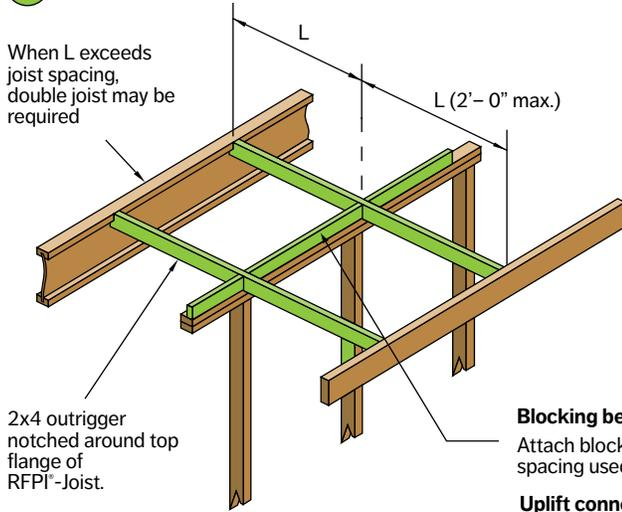
2x4 outrigger notched around top flange of RFPI®-Joist.
