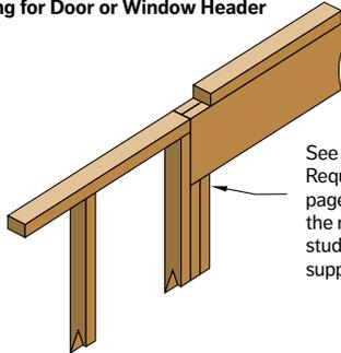
See "Bearing Length Requirements" on page 42 to determine the number of jack studs required to support header.
