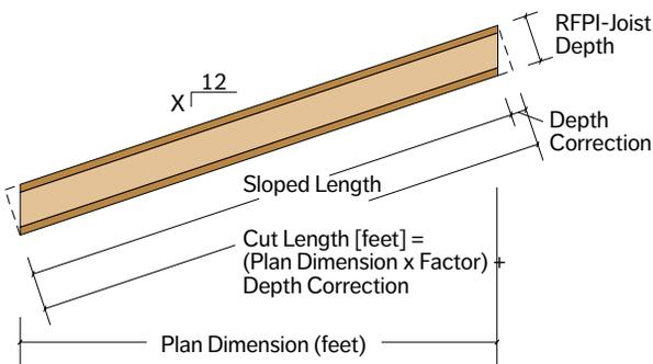
**ALONG-THE-SLOPE SPANS & CUTTING LENGTHS FOR SLOPED ROOFS**
