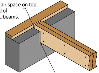
Provide moisture barrier between RigidLam LVL beams and concrete.
