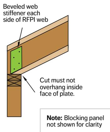
**2e RFPI®-JOISTS ON BEVELED PLATE**
