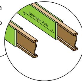
Use nailing pattern shown for Method 1 with opposite face nailing offset by 3"
