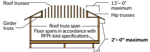
For hip roofs with the hip trusses running parallel to the cantilevered floor joists, the I-joist reinforcement requirements for a span of 26' may be used.
