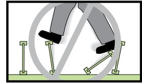
Do not allow workers to walk on I-joists or LVL beams until they are fully installed and braced, or serious injuries can result.
