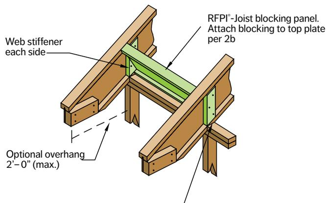
Birdsmouth cut RFPI®-Joist to provide full bearing for bottom flange. Cut must not overhang inside face of plate.
