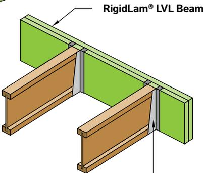
Top- or face-mounted hanger installed per hanger manufacturer's recommendations
