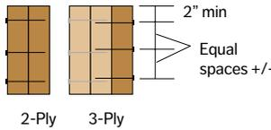
For 14", 16" or 18" deep members, nail plies together with 3 rows of 16dx3-1/2" com. nails at 12" o.c. (add 1 row for 16d sinkers).
