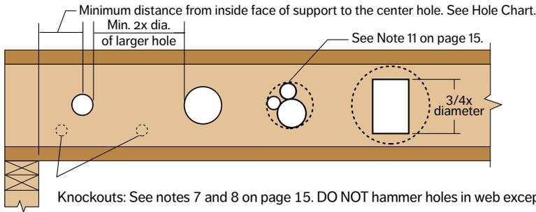
**RFPI-JOIST TYPICAL HOLES** - See "HOW TO USE HOLE CHART" below and "Rules for Cutting Holes in RFPI Joists" on page 15
