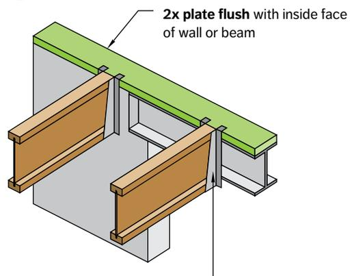
Top-mounted hanger installed per hanger manufacturer's recommendations
