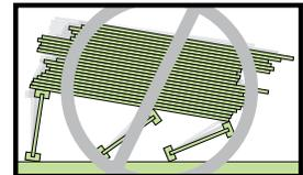
Never stack building materials over unbraced I-joists. Stack only over braced beams or walls.
