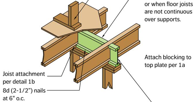
RFPI® blocking panel factored vertical load transfer = 2,900 plf maximum -or- RigidRim Rimboard (see Page 34 for design properties)
