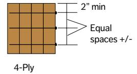
The recommended fastener spacing is two rows at 24" o.c. for up to and including 16" deep members, and 3 rows at 24" o.c. for members up to and including 24" deep. If the fastener point penetrates a minimum of 75% of the 4th ply, they may be applied from one side of the beam; otherwise, the fasteners must be applied from both sides and staggered.
