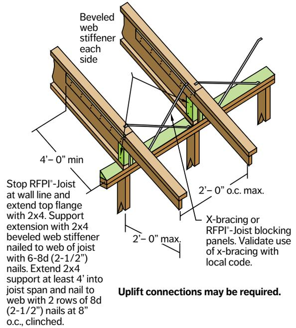
Stop RFPI®-Joist at wall line and extend top flange with 2x4. Support extension with 2x4 beveled web stiffener nailed to web of joist with 6-8d (2-1/2") nails. Extend 2x4 support at least 4' into joist span and nail to web with 2 rows of 8d (2-1/2") nails at 8" o.c., clinched.
