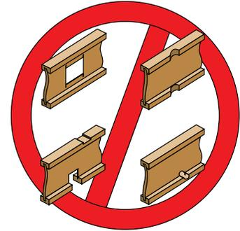
**Never** drill, cut or notch the flange, or over-cut the web. Holes in webs should be cut with a sharp saw. For rectangular holes, avoid over-cutting the corners, as this can cause unnecessary stress concentrations. Slightly rounding the corners is recommended. Start the rectangular hole by drilling a 1"-diameter hole in each of the four corners and then make the cuts between the holes to minimize damage to the I-joist.
